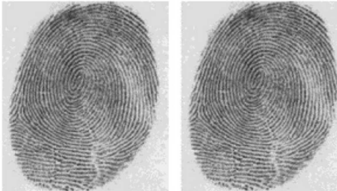
Fig. 5. An FBI-digitized left thumb fingerprint. The image on the left is the original; the one on the right is reconstructed from a 26:1 compression. These images can be retrieved by anonymous FTP at ftp.c3.lanl.gov (128.165.21.64) in the directory pub/WSQ/print_data . (Courtesy Chris Brislawn, Los Alamos National Laboratory.)
