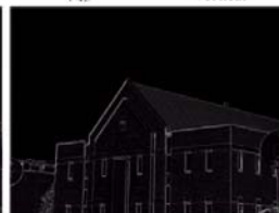
FIGURE 10.12 Diagonal edge detection. (a) Result of using the mask in Fig. 10.9(c). (b) Result of using the mask in Fig. 10.9(d). The input in both cases was Fig. 10.11(a).
