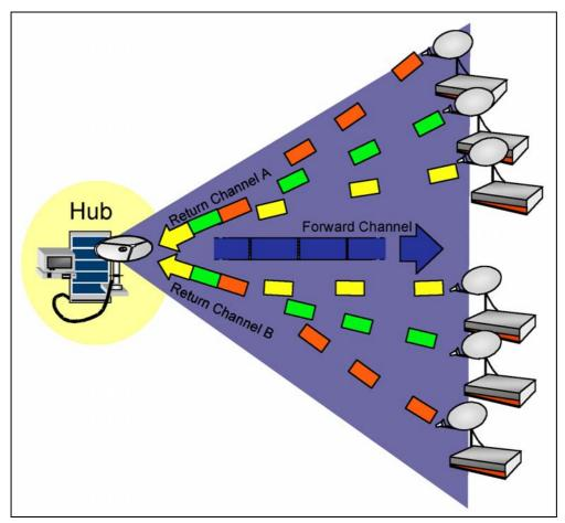
Fig. 2.2 Two-way communications via forward and return links.
