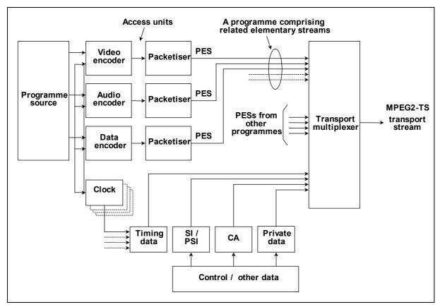
Fig.2.12 Baseband processing of programme material to an MPEG2 transport stream. Key: CA: Conditional Access, PES: Packetised Elementary Stream (long streams, for local use only), PSI: Programme- Specific Information, SI: Service Information, TS: Transport Stream.
