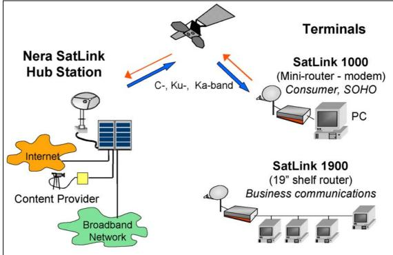
Fig. 2.1 SatLink DVB-RCS system block diagram.
