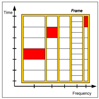
Fig. 2.3 Dynamic slot MF-TDMA.
