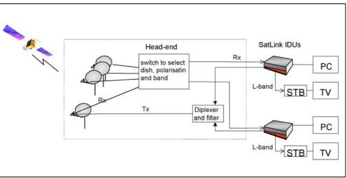
Fig. 3.4 SMATV head-end facilities are easily supported over satellite.
