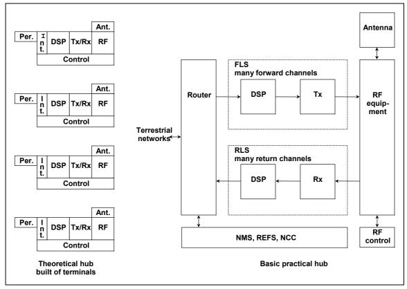
Fig. 1.15 The basic practical Hub station resembles the theoretical station built of many Terminals.
