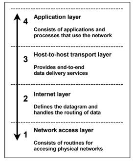
Fig. 1.2 Four-layer TCP/IP model.
