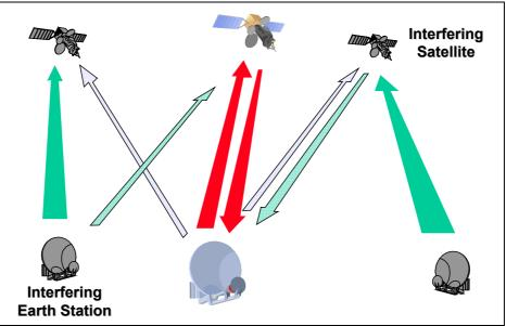
Fig. 1.23 Interference, from other Earth Stations upon the uplink and from the downlinks from other satellites, degrades communication and therefore must be taken into account in link budgets.
