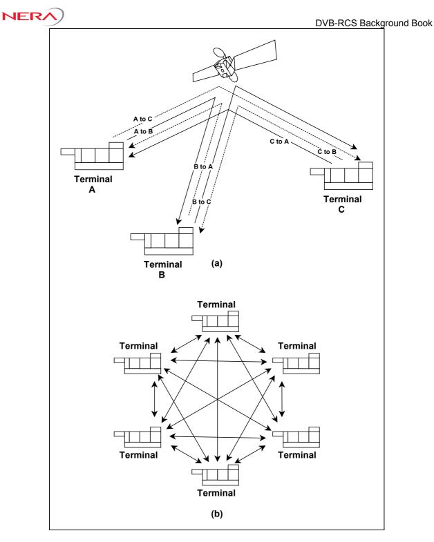
Fig. 1.12 Typical mesh network with three Terminals communicating via the satellite (a) and an overall mesh of communications between the Terminals of a six-station network (b).
