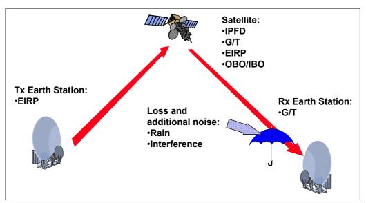
Fig. 1.22 Link budget parameters.
