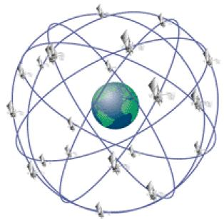
Fig. 2.5 Global Positioning System (GPS) satellite constellation, with 24 satellites in six orbital planes; each orbit is at an altitude of about 20,200 km above the surface of the Earth. Drawing from the GPS pages of the Federal Aviation Administration website at gps.faa.gov/index.htm
