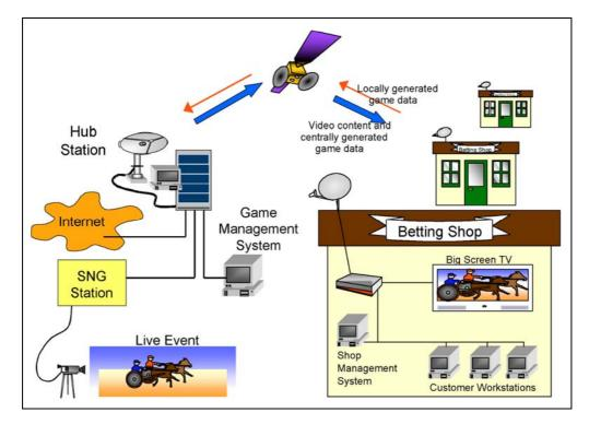
Fig. 3.3 A Betting Shop Network is typical of a VPN easily supported by satellite.
