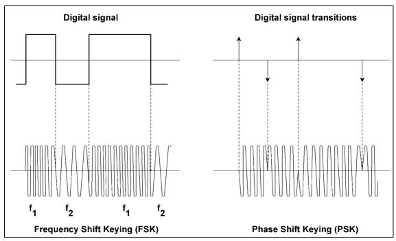
Fig. 1.17 Basic actions of frequency shift keying and phase shift keying.
