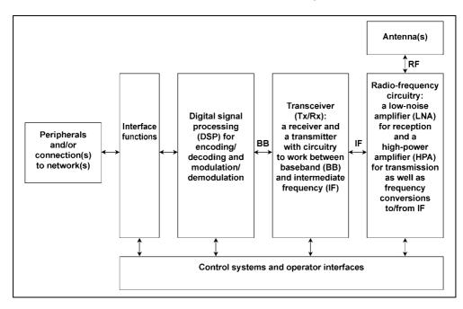
Fig. 1.10 All digital radio communications stations consist of seven basic "building blocks" that interwork between BaseBand (BB), Intermediate Frequency (IF) and Radio Frequency (RF).
