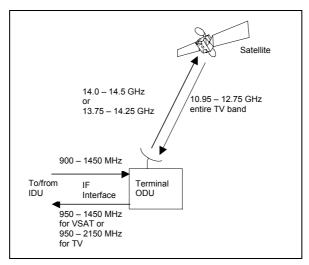
Fig. 1.26 Radio frequency bandwidths at a Terminal in a Ku-band system.
