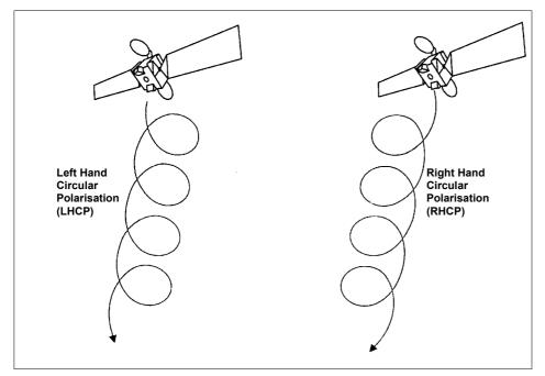
Fig. 1.27 Left-hand circular and right-hand circular polarisations.
