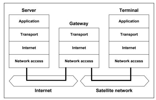
Fig. 1.6 A gateway providing TCP/IP over satellite processes data up to the Transport layer to provide Internet-quality connections to Terminals.
