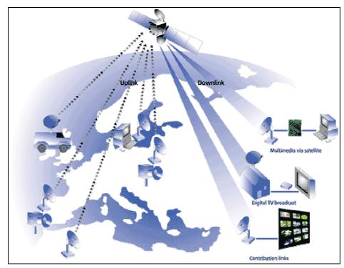
Fig. 1.9 Skyplex regenerative transponder system [drawing from Eutelsat website at <a href="http://www.eutelsat.org/">http://www.eutelsat.org/</a>].
