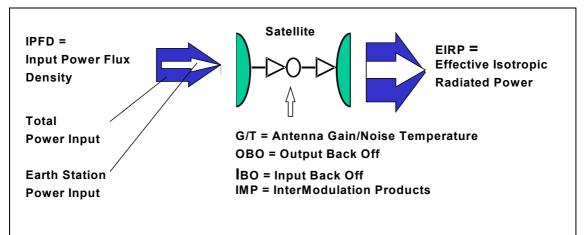
Fig. 1.21 Satellite transponder parameters.
