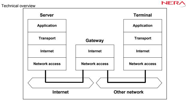
Fig. 1.5 Basic network-to-network flow of data between an Internet server and a user Terminal connected to another network.
