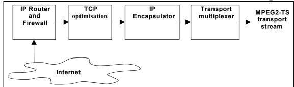
Fig. 2.14 Baseband processing of IP material to an MPEG2 transport stream.
