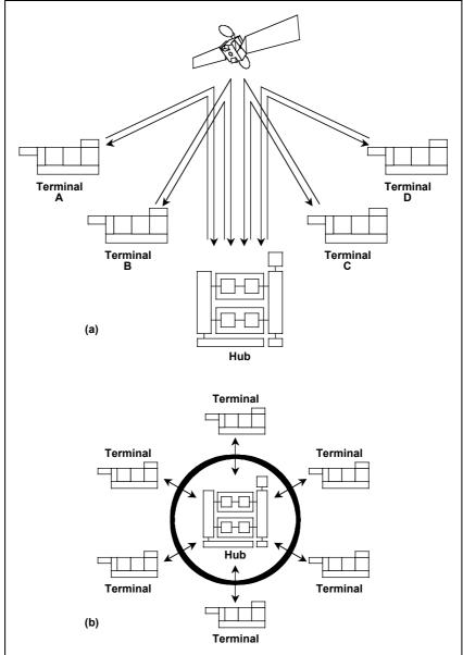
Fig. 1.13 Typical star network with four Terminals communicating via a central Hub station (a) and overall star of communication channels between the Terminals in a six-station network (b).
