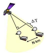
Fig. 2.4 Terminals are located at different places, so the uplink transmission times to and from them vary.
