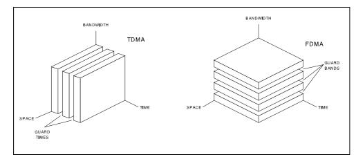
Fig. 1.7 Time domain and frequency domain multiple access. Guard times in TDMA and guard bands in FDMA prevent interference between adjacent signals. However, in system design, both guard times and guard bands are minimised, because they carry no information and consequently waste satellite resources.
