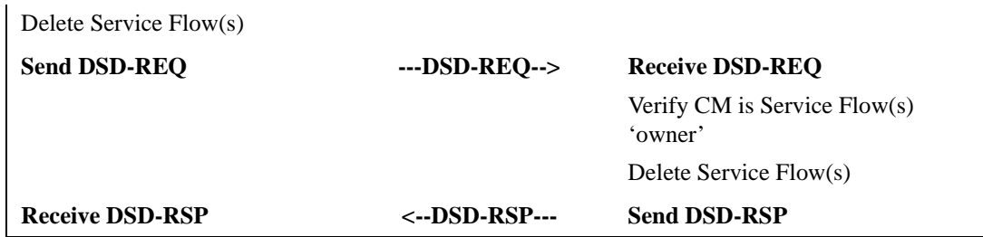
Figure 9-50. Dynamic Service Deletion Initiated from CM
