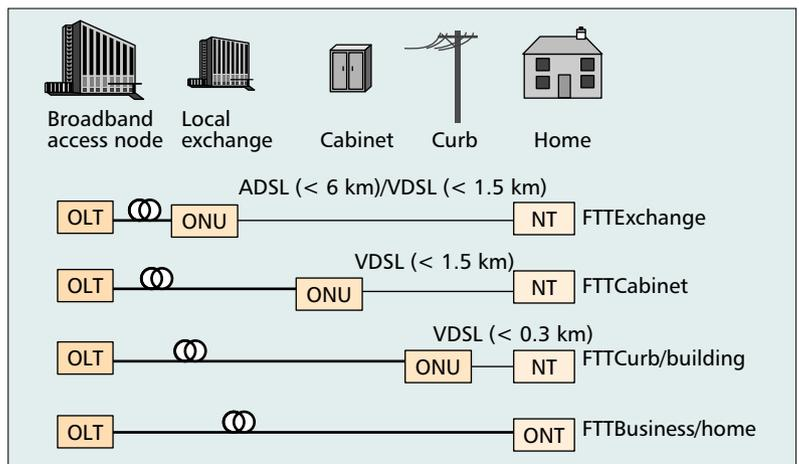
■ **Figure 2.** Fiber to the x topologies.
