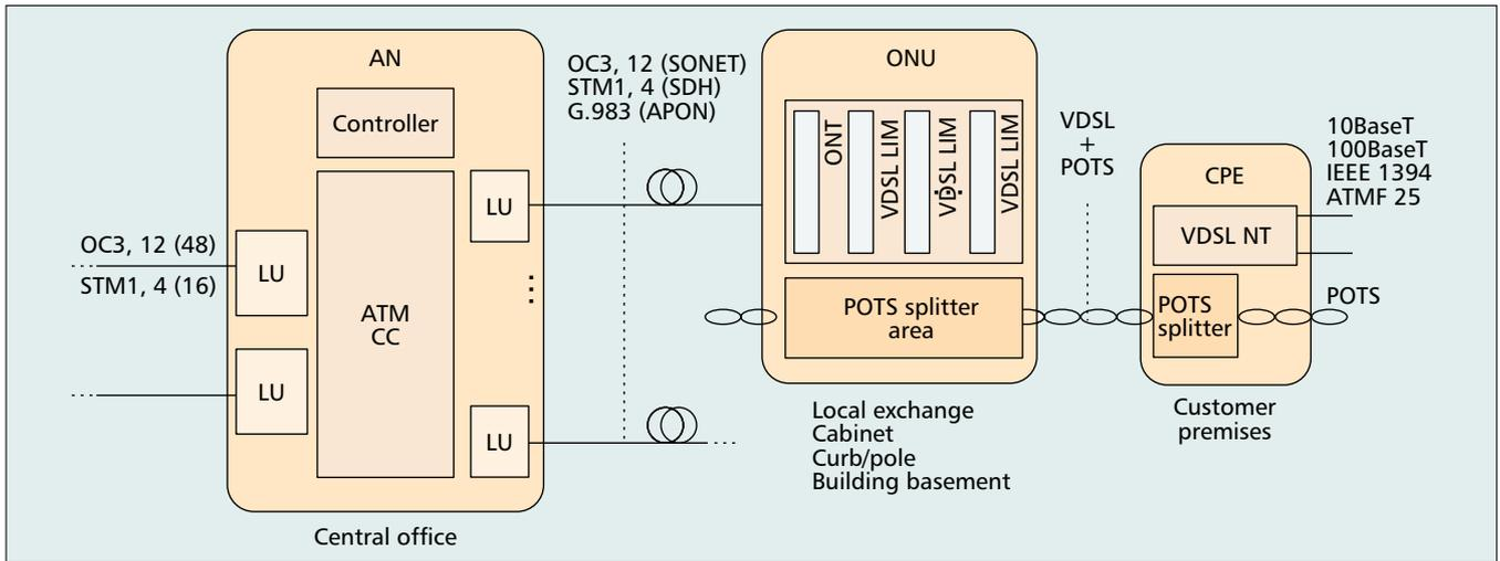
■ **Figure 1.** The general network model for VDSL deployment.
