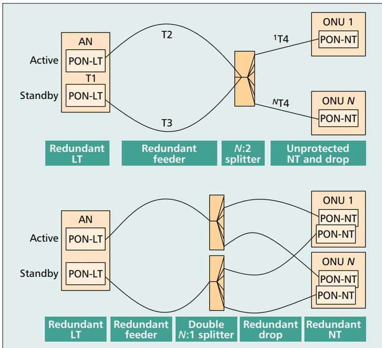
■ Figure 5. Root redundancy and full redundancy of APON.
