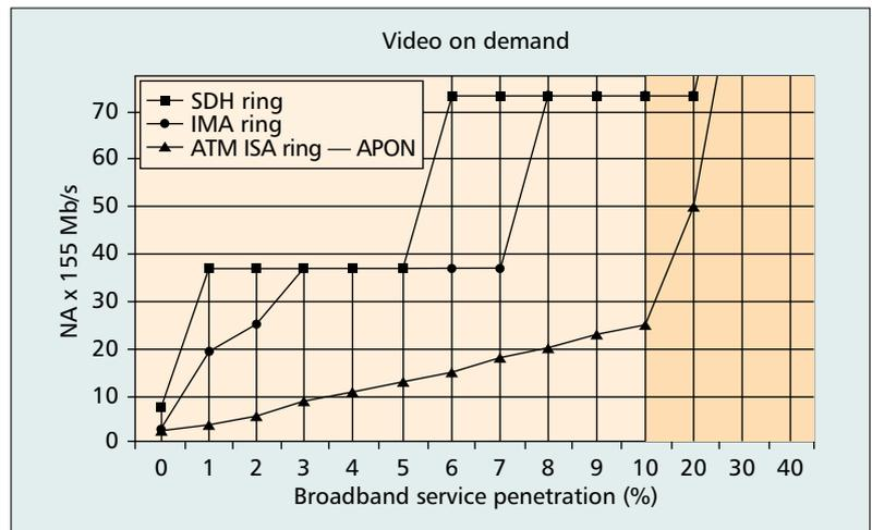
Figure 6. A comparison of APON with various multiplexing approaches on SDH rings.
