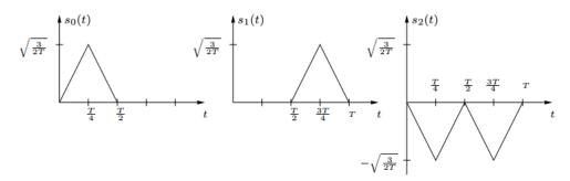
They are used to transmit symbols in a communication system with n repeaters. Each repeater estimates the transmitted symbol from the previous transmitter and retransmits it. Assume ML detection in all receivers.
