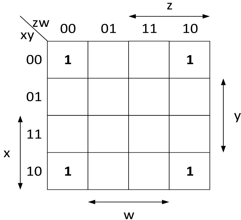
$$\begin{aligned}F(x, y, z, w) &= x'y'z'w' + x'y'zw' + xy'z'w' + xy'zw' \\&= x'y'w'(z' + z) + xy'w'(z' + z) \\&= x'y'w' + xy'w' = (x' + x)y'w' = y'w'\end{aligned}$$
