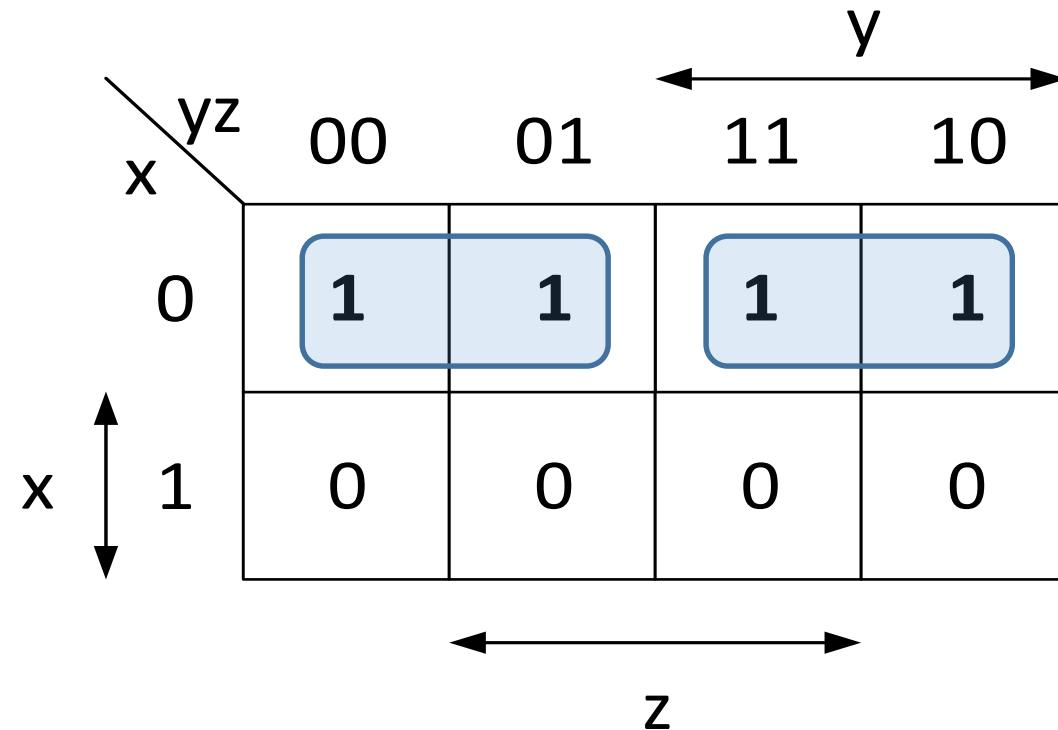
$$F = x'y' + x'y = x'(y' + y) = x'$$
