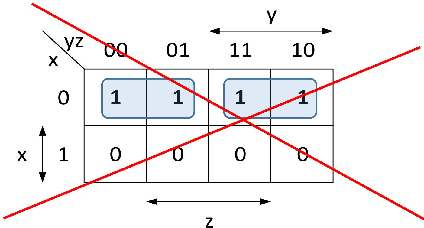
$$F = x'y' + x'y = x'(y' + y) = x'$$
