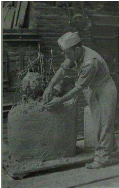
2.7 Outer layer of clay investment mold, coarser and drier than the inner layer, is built up over the model and gate system. Courtesy of Alison Frantz.
