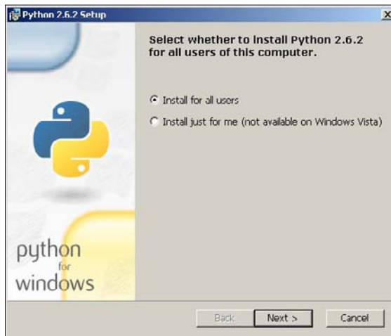
Figure 17-3: Python can be limited to a single user or it can be open to all users.
