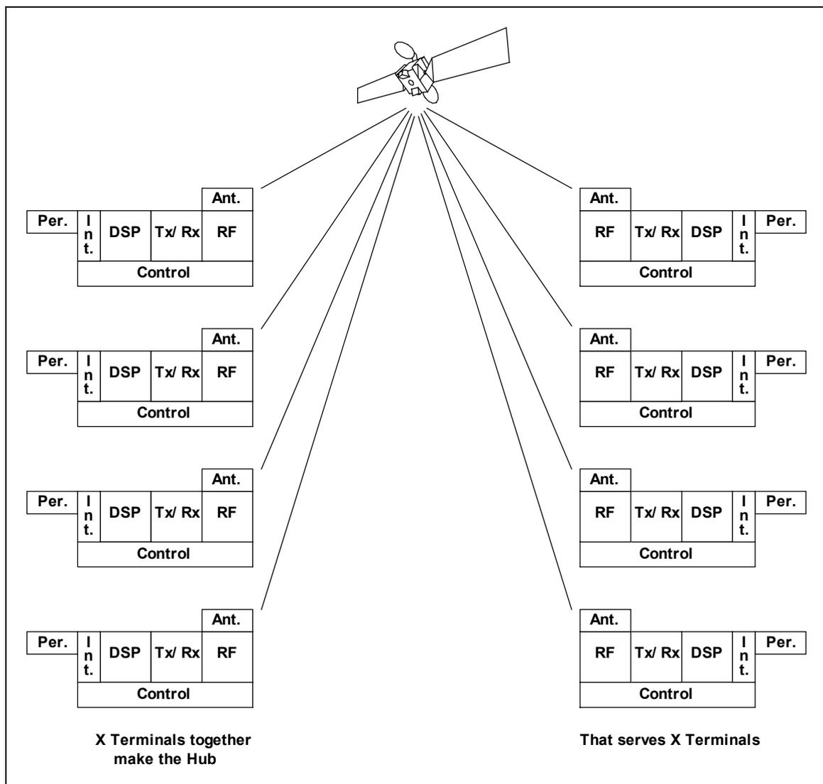
**Fig. 1.14 Theoretically, a Hub station might be built using many Terminals.**
