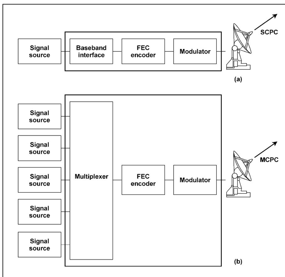
**Fig. 1.19 MCPC and SCPC transponder access. DVB-S is designed primarily for MF-TDMA, which is a variety of MCPC.**
