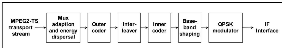
Fig. 2.15 Functional block diagram of digital signal processing using concatenated coding in a transmitter. The functions are reversed in a receiver.
