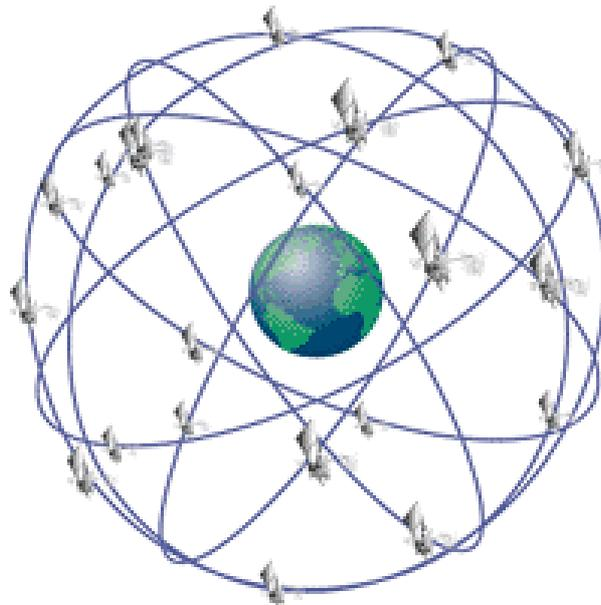
**Fig. 2.5 Global Positioning System (GPS) satellite constellation, with 24 satellites in six orbital planes; each orbit is at an altitude of about 20,200 km above the surface of the Earth. Drawing from the GPS pages of the Federal Aviation Administration website at [gps.faa.gov/index.htm](http://gps.faa.gov/index.htm)**
