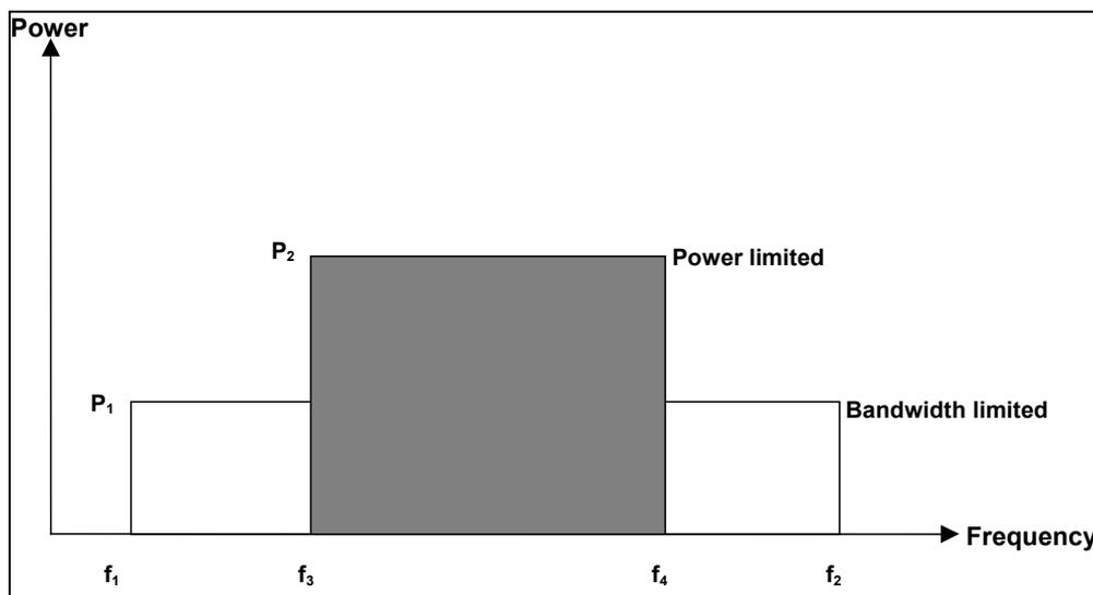
**Fig. 1.20** A transponder is limited in bandwidth and power. If its maximum bandwidth,  $f_2 - f_1$ , is used, it is said to be bandwidth limited and can transmit at power  $P_1$ . If its maximum power,  $P_2$ , is used, it is said to be power limited and can transmit over a bandwidth  $f_4 - f_3$ .
