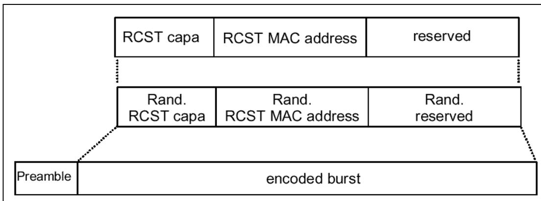
**Fig. 2.6 Common Signalling Channel (CSC) burst format, from Fig. 9 in ETSI EN 301 790 [15].**
