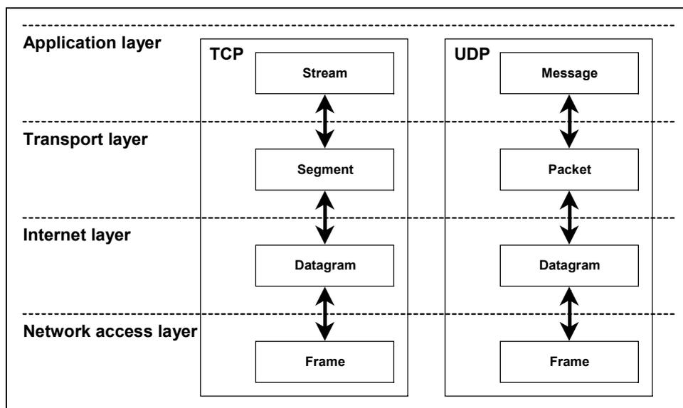
Fig. 1.4 Common terminology for data at various layers.
