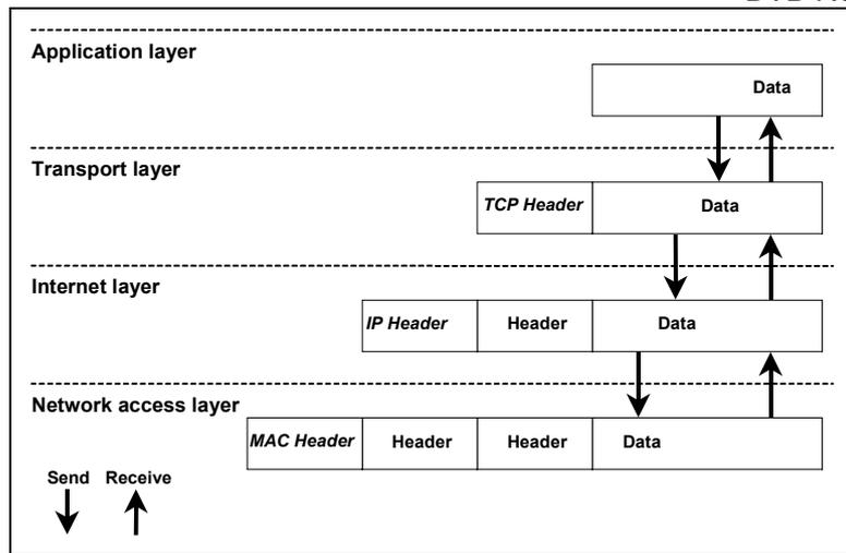
Fig. 1.3 Headers are added to data sent and removed from data received, as the data are passed between layers.
