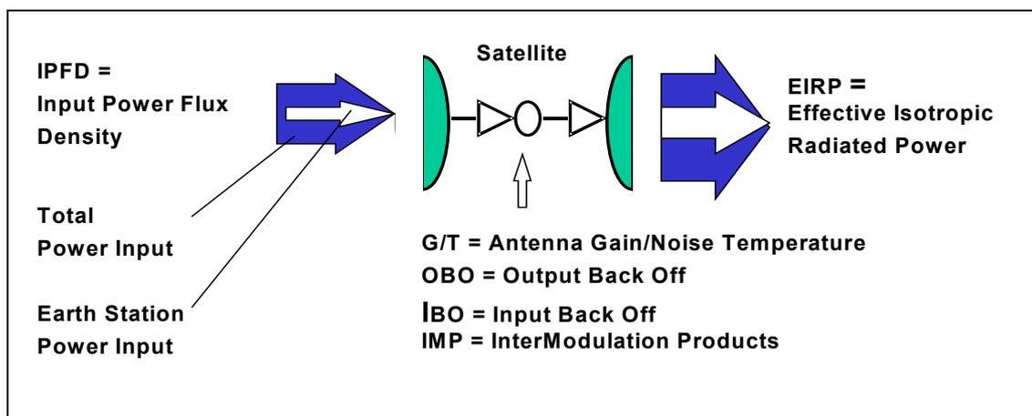
**Fig. 1.21** Satellite transponder parameters.
