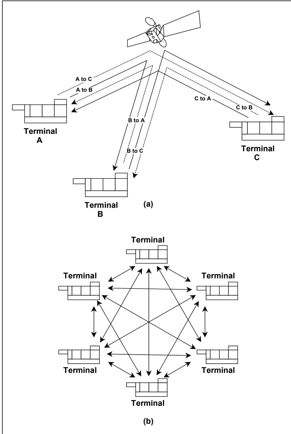
Fig. 1.12 Typical mesh network with three Terminals communicating via the satellite (a) and an overall mesh of communications between the Terminals of a six-station network (b).
