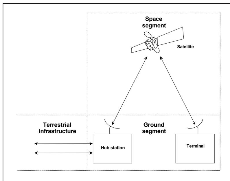
**Fig. 1.8 Like all satcom systems, the basic broadband over satellite system has three parts.**
