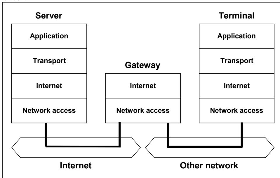
Fig. 1.5 Basic network-to-network flow of data between an Internet server and a user Terminal connected to another network.
