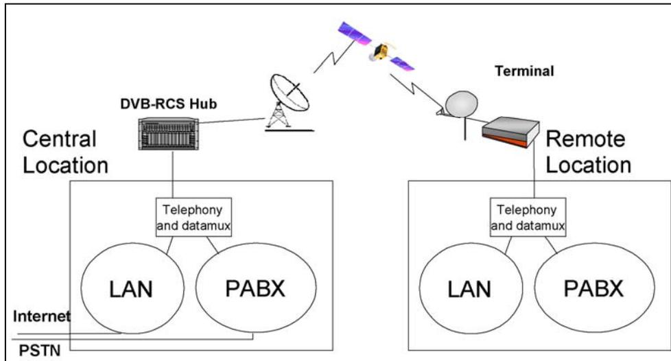
Fig. 3.1 Satellite links can bring telecommunications to locations previously under-served.
