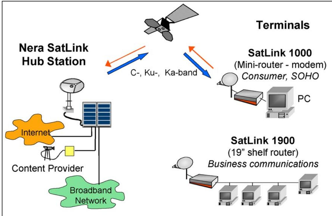
**Fig. 2.1 SatLink DVB-RCS system block diagram.**
