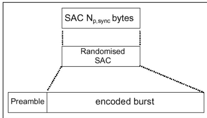
**Fig. 2.8 Synchronisation (SYNC) burst format, from Fig. 7 in ETSI EN 301 790 [15].**
