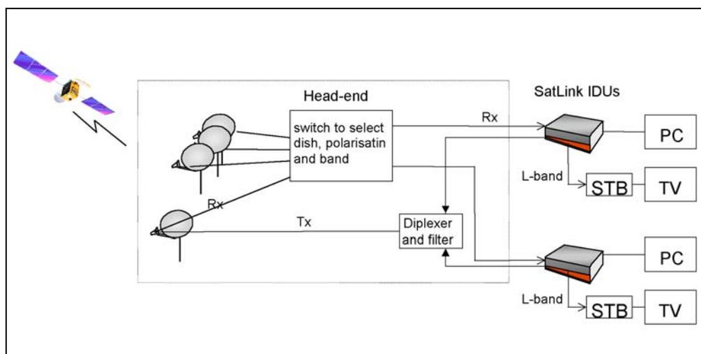
**Fig. 3.4 SMATV head-end facilities are easily supported over satellite.**
