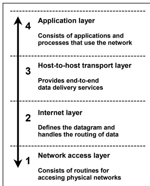
Fig. 1.2 Four-layer TCP/IP model.
