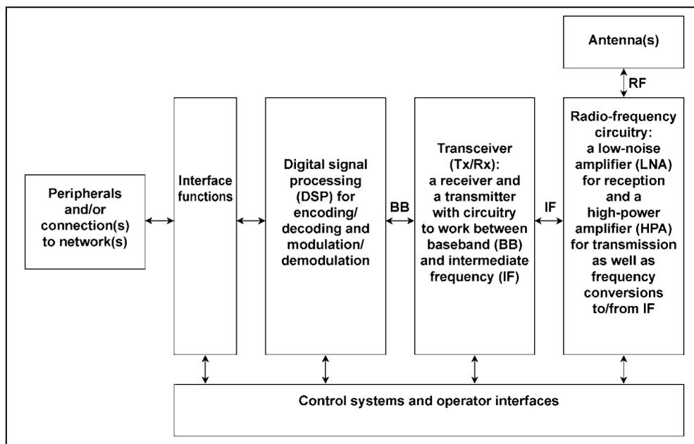
**Fig. 1.10 All digital radio communications stations consist of seven basic “building blocks” that interwork between BaseBand (BB), Intermediate Frequency (IF) and Radio Frequency (RF).**
