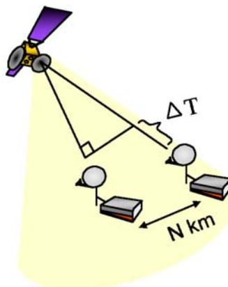
Fig. 2.4 Terminals are located at different places, so the uplink transmission times to and from them vary.
