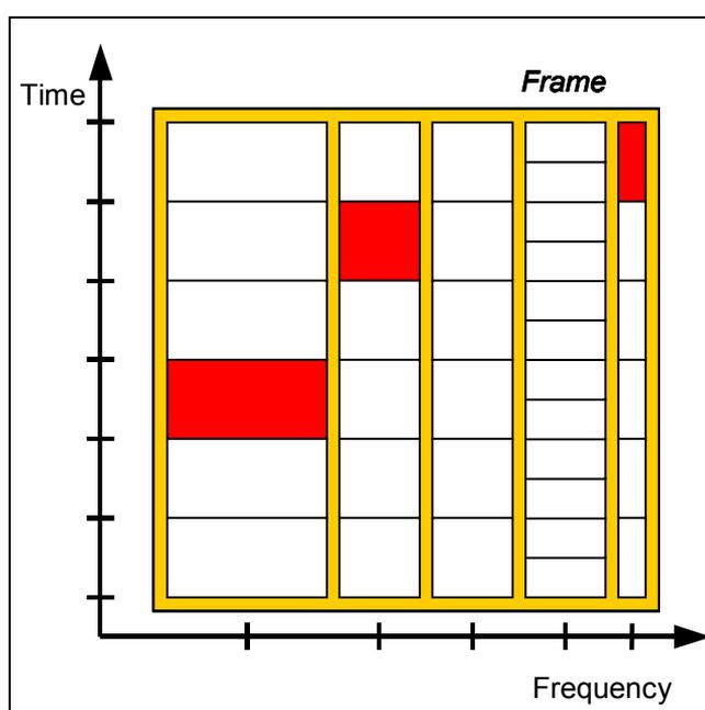
**Fig. 2.3 Dynamic slot MF-TDMA.**
