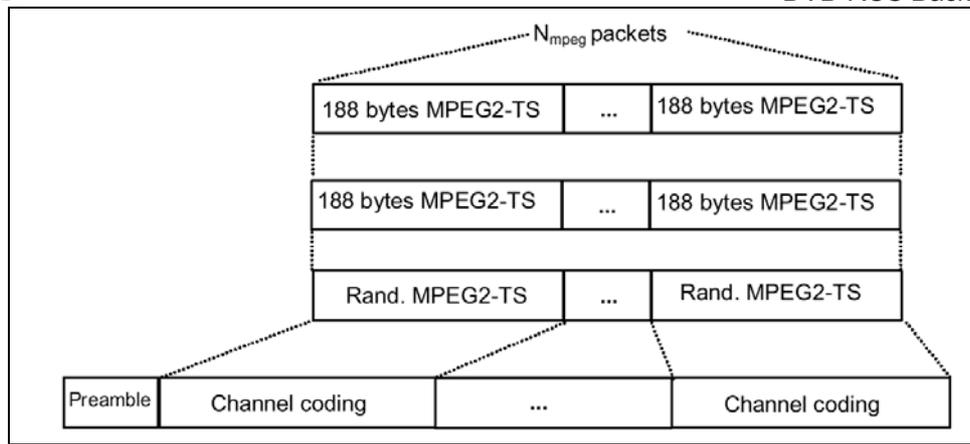
Fig. 2.10 Traffic (TRF) burst format using MPEG2 wrappers, from Fig. 6 in ETSI EN 301 790 [15].
