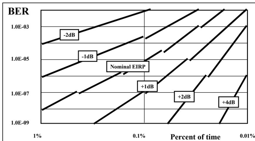
**Fig. 1.24 Probability of maximum BER as a function of EIRP, including loss due to rain attenuation.**
