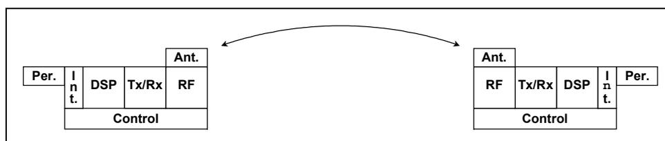
**Fig. 1.11 Basic station communications.**
