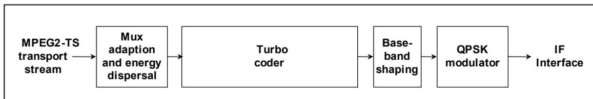
Fig. 2.16 Functional block diagram of digital signal processing using Turbo coding in a transmitter. The functions are reversed in a receiver.
