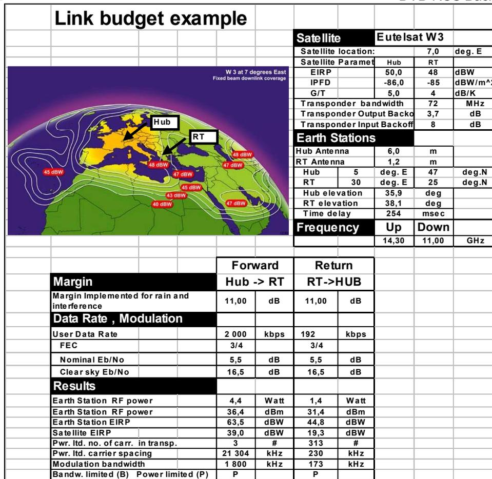
Fig. 1.25 Typical link budget, for EBU Data Distribution System. The cases shown are power limited in the transponder.
