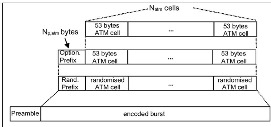
Fig. 2.11 Traffic (TRF) burst format using ATM wrappers, from Fig. 5 in ETSI EN 301 790 [15].
