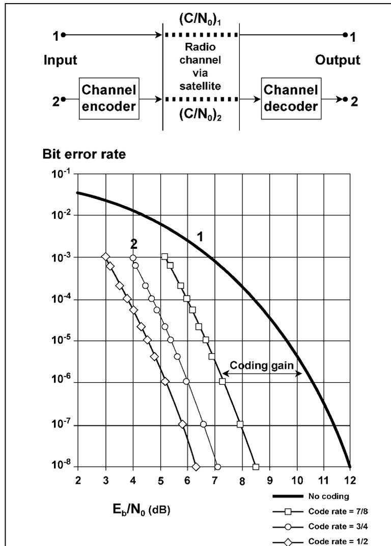
**Fig. 1.16 Coding performance can be assessed by comparing the Bit Error Rate (BER) of coded links to that of an uncoded link. The curves shown are for convolutional coding and a typical Viterbi decoder at the receiver. Figure adapted from Fig. 5.35 in “VSAT Networks” [12]**
