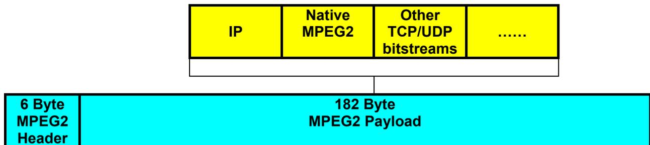
Fig. 2.9 Digital wrapping in which traffic having various protocols is enclosed in MPEG2 packets.
