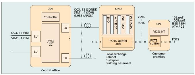
**Figure 1.** *The general network model for VDSL deployment.*
