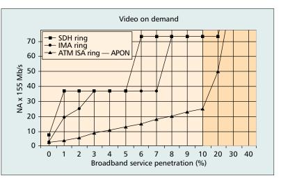
**Figure 6.** *A comparison of APON with various multiplexing approaches on SDH rings.*
