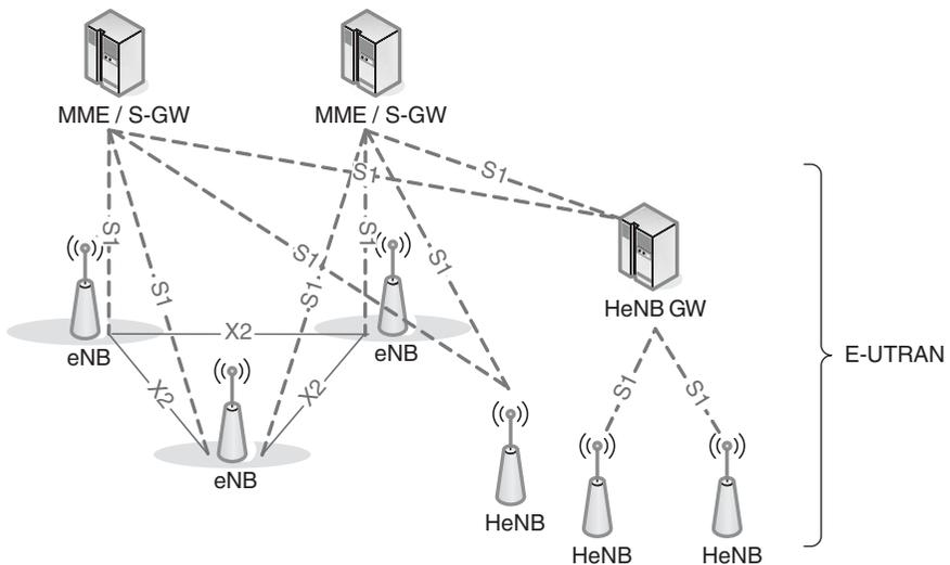
**Figure 9.5** Architecture with HeNBs. Reproduced by permission of © 2010 3GPP. Further use is strictly prohibited.
