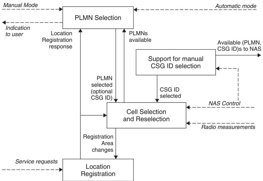
**Figure 11.1** IDLE Mode Process. Reproduced by permission of © 2010 3GPP. Further use is strictly prohibited.
