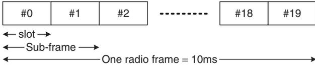
**Figure 10.1** Type-1 Frame structure. Reproduced by permission of © 2010 3GPP. Further use is strictly prohibited.
