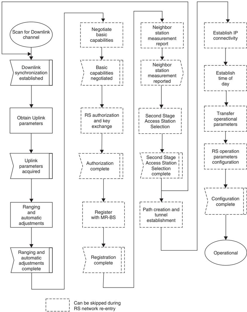
**Figure 5.2** Network Entry and Initialization flowchart for IEEE 802.16-2009. An adaptation from Figure 65a, page 102 in 16j-2009 “RS Initialization”. Reproduced by permission of © 2009 IEEE.
