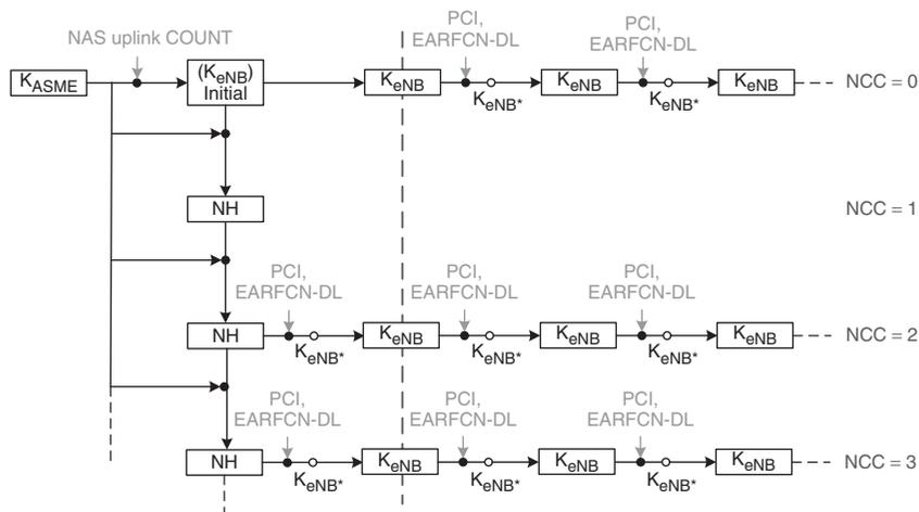
**Figure 14.4** Key Handling during Handover. Reproduced by permission of © 2010 3GPP. Further use is strictly prohibited.
