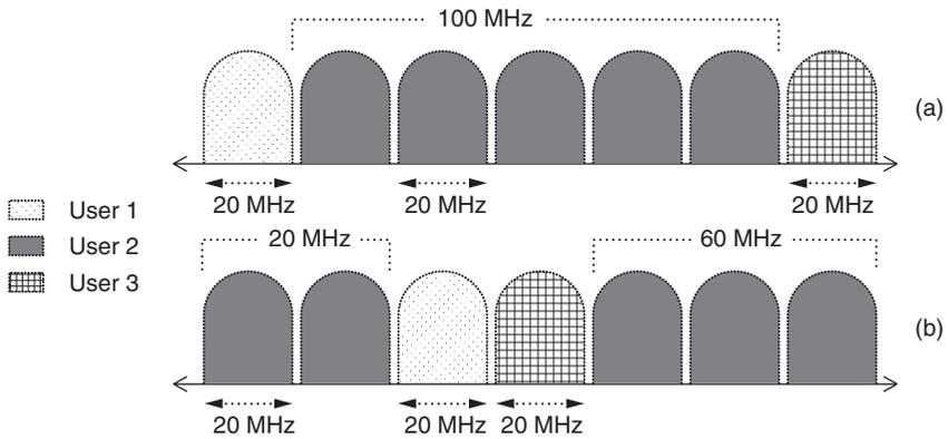
**Figure 2.6** Carrier aggregation. (a) Contiguous carrier aggregation and (b) noncontiguous carrier aggregation.
