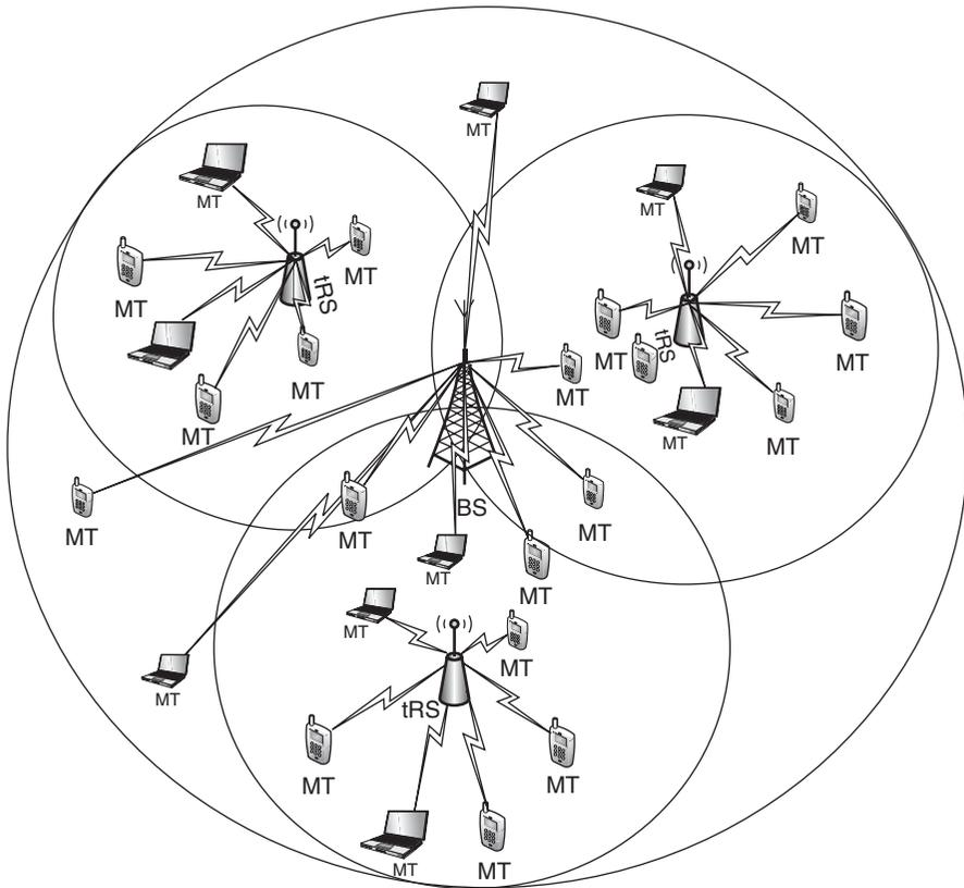
**Figure 2.8** Network where transparent RSs are used for capacity enhancement.
