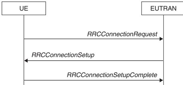
**Figure 11.4** A successful RRC Connection Establishment. Reproduced by permission of © 2010 3GPP. Further use is strictly prohibited.
