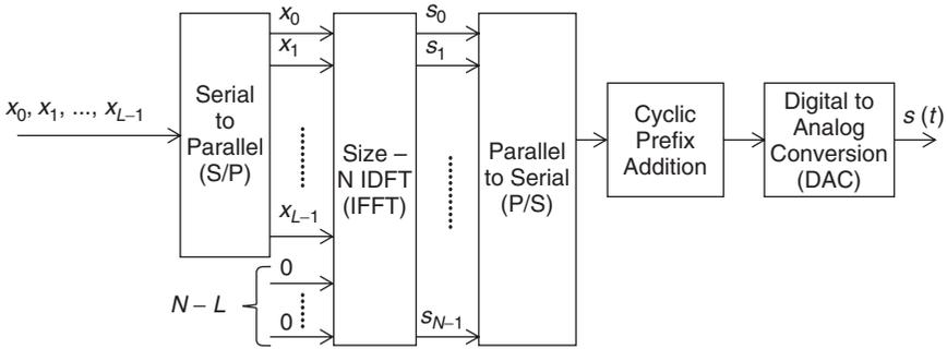
**Figure 2.1** OFDM modulation using the IFFT.
