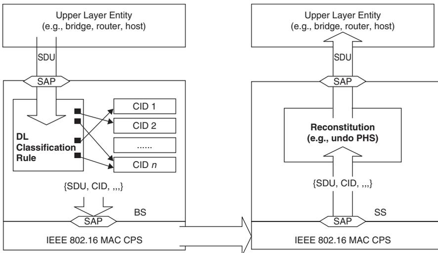
**Figure 6.1** Classification and CID mapping (BS-to-MS). Reproduced by permission of © 2009 IEEE.
