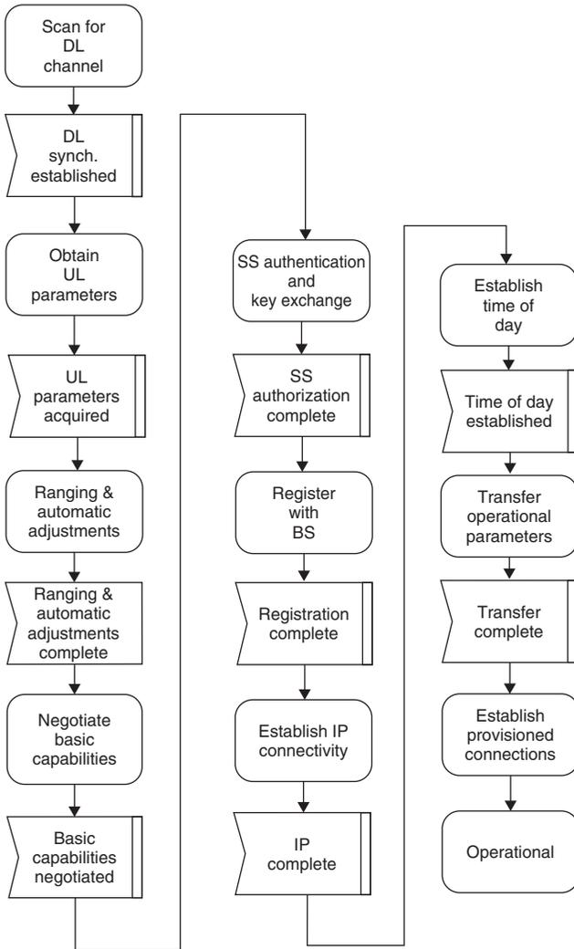
**Figure 5.1** Network Entry and Initialization flowchart for IEEE 802.16-2009. Reproduced by permission of © 2009 IEEE.
