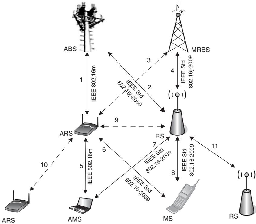
**Figure 3.5** An example deployment of an IEEE 802.16m showing different types of links possible between legacy (IEEE 802.16-2009) and advanced IEEE 802.16m network elements. Reproduced by permission of © 2009 IEEE.
