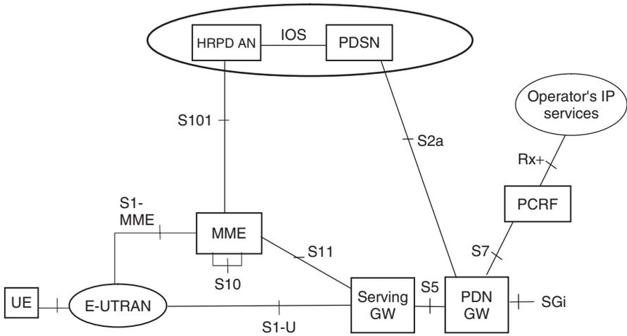
**Figure 16.2** Architecture for optimized handover between mobile WiMAX and 3GPP2.
