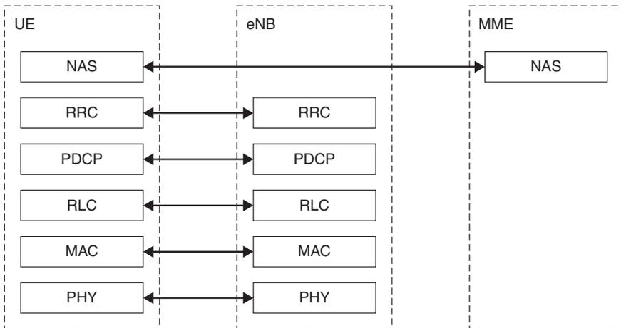
**Figure 9.4** LTE Control Plane. Adaptation. Reproduced by permission of © 2010 3GPP. Further use is strictly prohibited.
