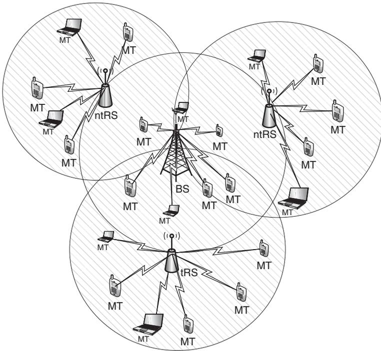
**Figure 2.9** Network where non-transparent stations are used for capacity enhancement.
