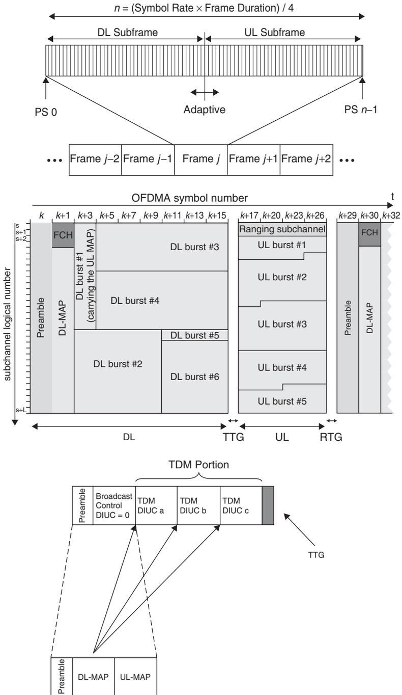
**Figure 4.1** OFDMA and OFDM frame structure, TDD operation mode. Reproduced by permission of © 2009 IEEE.
