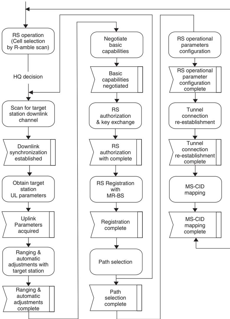
**Figure 7.2** Flowchart for the mobile relay station handover process. Reproduced by permission of © 2009 IEEE.
