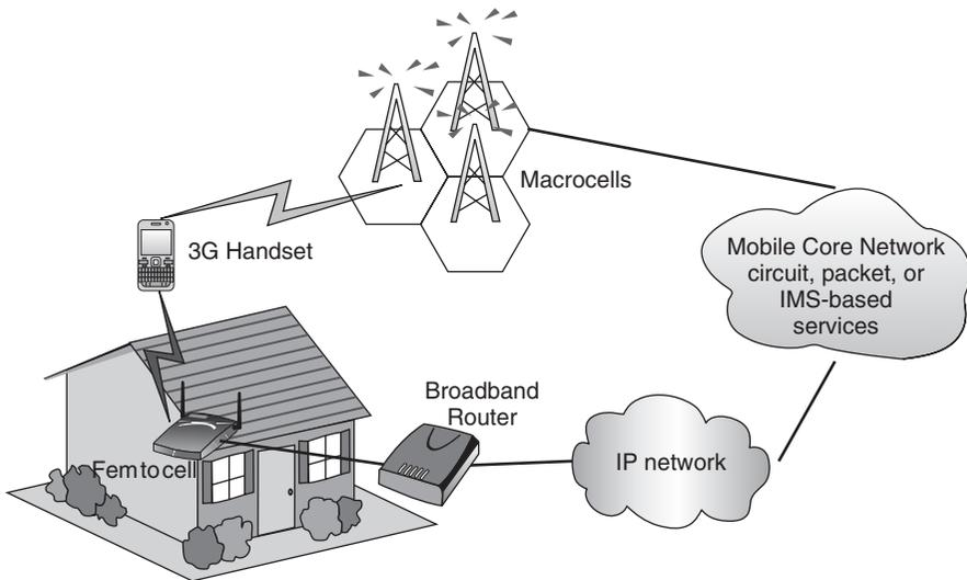
**Figure 2.10** An example of a femtocell setup.
