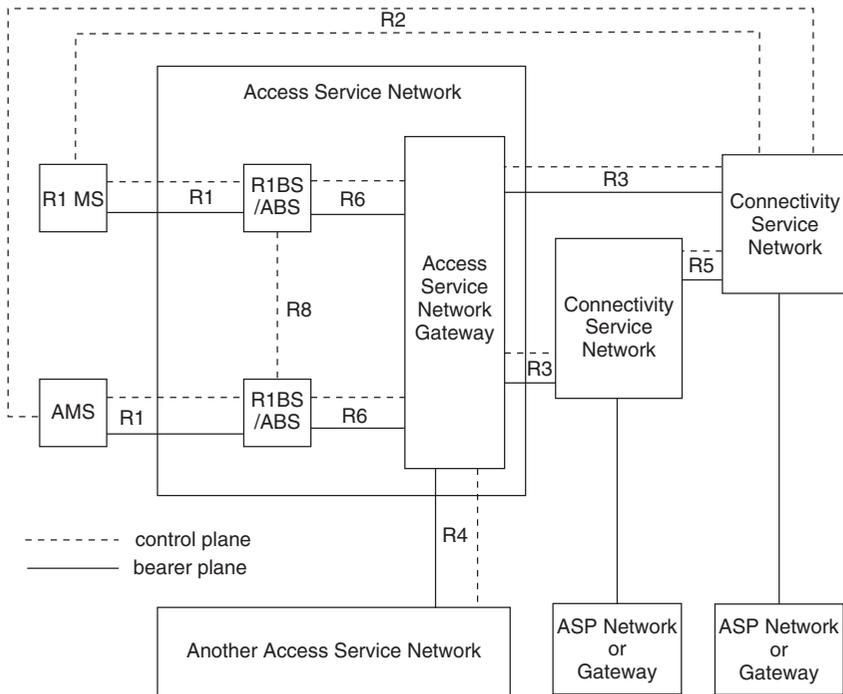
**Figure 3.4** The IEEE 802.16m network reference model. Reproduced by permission of © 2009 IEEE.
