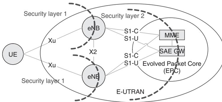
**Figure 14.1** First and second security layers in LTE. Reproduced by permission of © 2009 3GPP. Further use is strictly prohibited.
