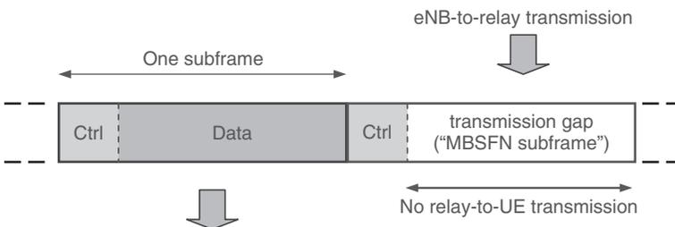
**Figure 12.4** Downlink resource partitioning for Inband-connection. Reproduced by permission of © 2010 3GPP. Further use is strictly prohibited.
