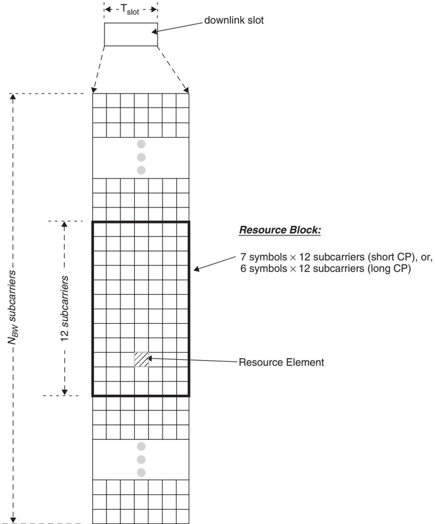
**Figure 10.3** The LTE Frame. Reproduced by permission of © 2010 3GPP. Further use is strictly prohibited.
