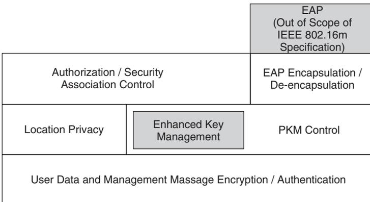
**Figure 8.2** Security Architecture in 16m. Reproduced by permission of © 2009 IEEE.
