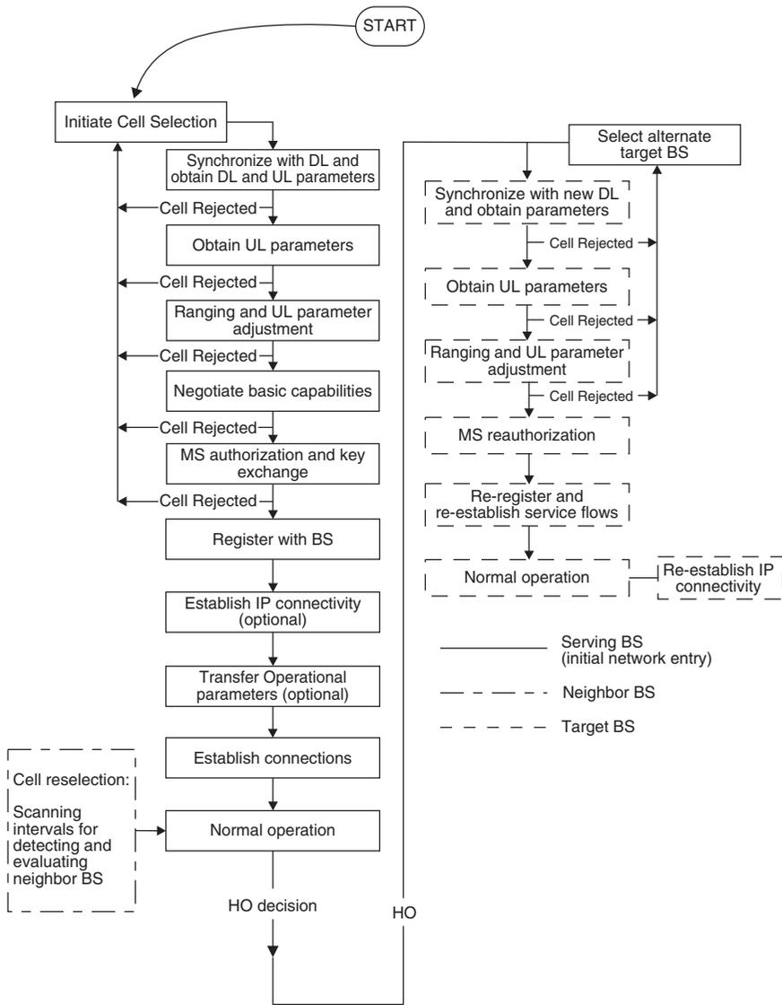
**Figure 7.1** Flow chart for handover process. Reproduced by permission of © 2009 IEEE.
