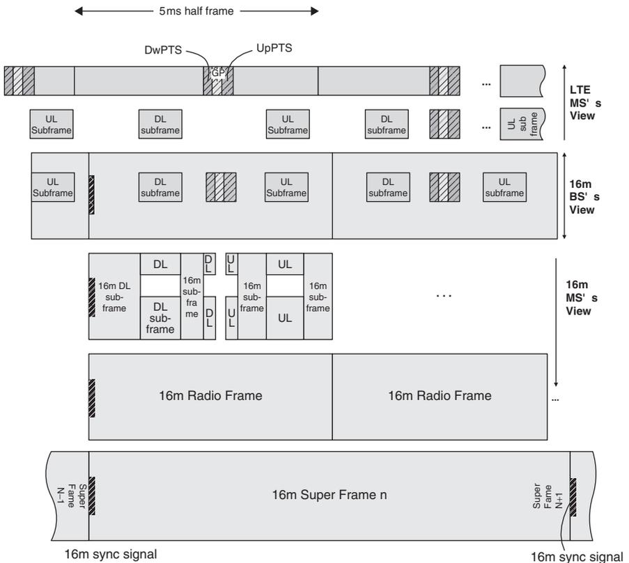
**Figure 16.1** Frame Structure Supporting LTE-TDD with IEEE 802.16m.
