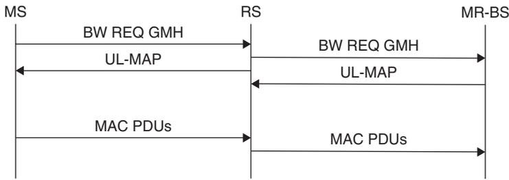
**Figure 6.6** An Example of a bandwidth request forwarded by the superordinate as soon as it is received from the subordinate. Reproduced by permission of © 2009 IEEE.
