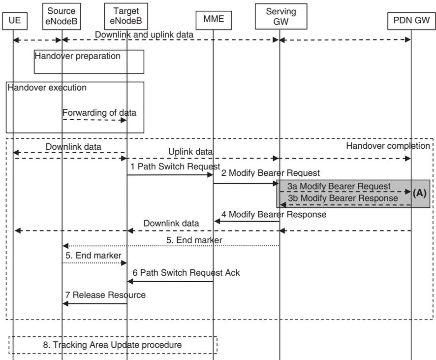
**Figure 13.5** X2-based handover without relocating serving GW. Reproduced by permission of © 2010 3GPP. Further use is strictly prohibited.
