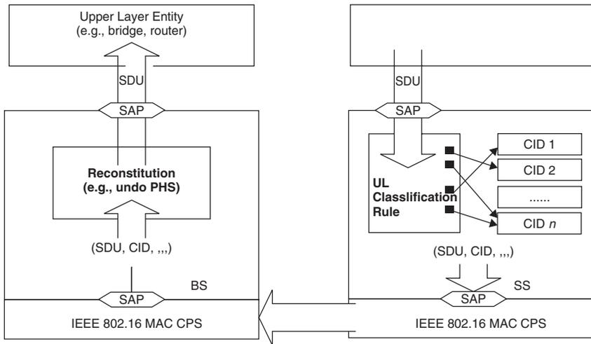
**Figure 6.2** Classification and CID mapping (MS-to-BS). Reproduced by permission of © 2009 IEEE.
