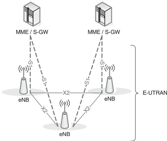
**Figure 9.1** Basic LTE and LTE-Advanced Architecture. Reproduced by permission of © 2010 3GPP. Further use is strictly prohibited.
