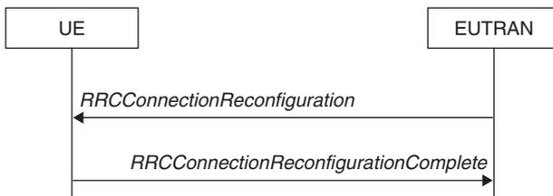
**Figure 11.5** A successful RRC Connection Reconfiguration. Reproduced by permission of © 2010 3GPP. Further use is strictly prohibited.
