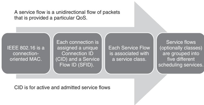
**Figure 6.4** Mapping traffic into transport connections, service flows and scheduling services.
