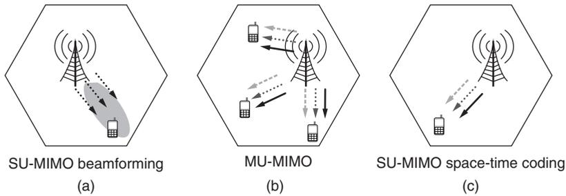
**Figure 2.7** Illustration of SU and MU MIMO systems.
