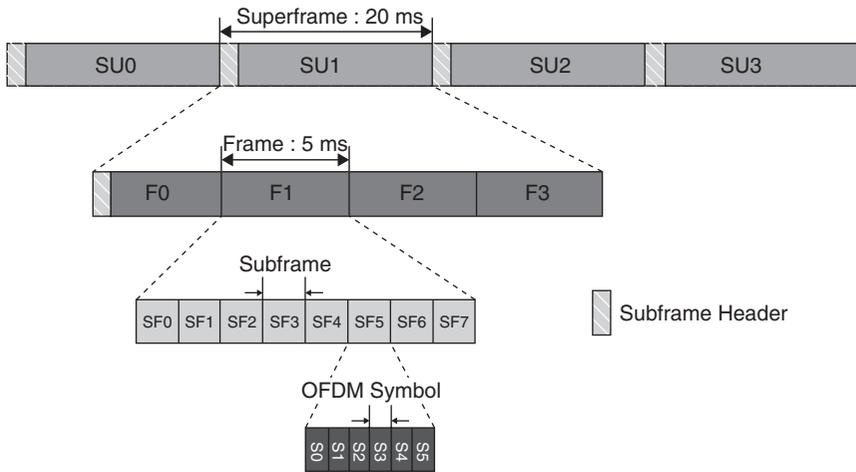
**Figure 4.7** IEEE 802.16m basic frame structure. Reproduced by permission of © 2009 IEEE.
