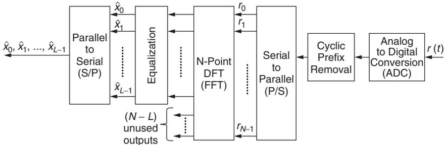
**Figure 2.2** OFDM demodulation.
