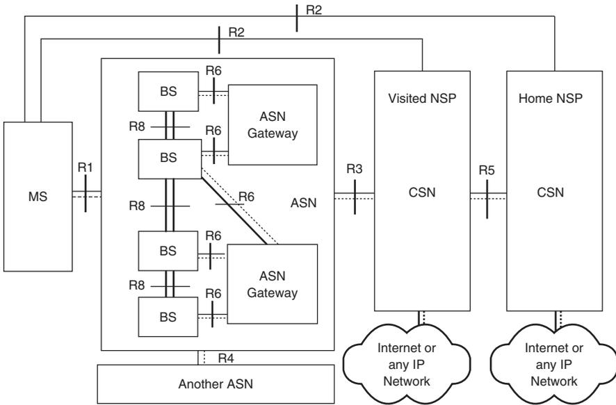
Figure 15.4 WiMAX Network Architecture.
