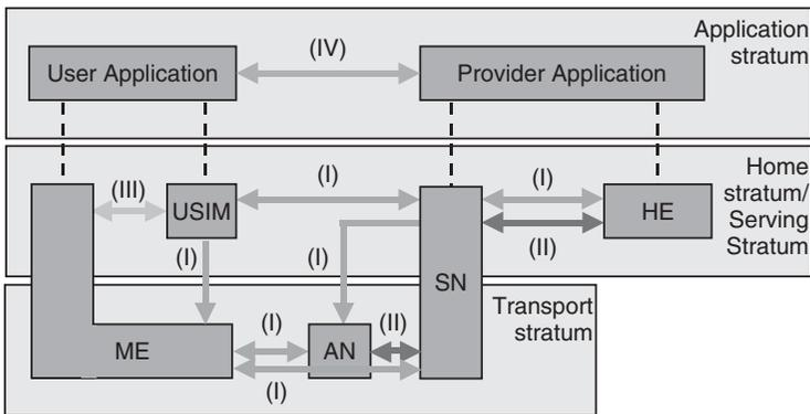
**Figure 14.2** Overview of LTE Security Architecture. Reproduced by permission of © 2010 3GPP. Further use is strictly prohibited.
