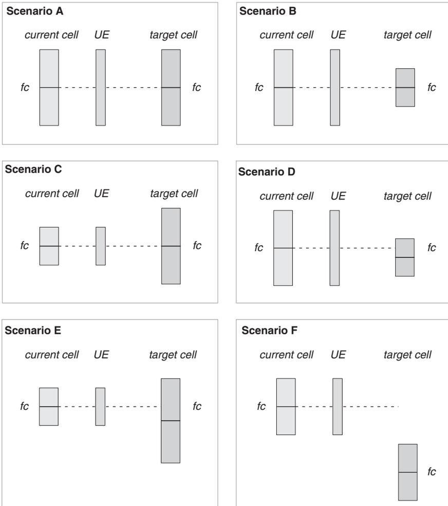
**Figure 13.2** Inter and intra-frequency measurement scenarios. Reproduced by permission of © 2010 3GPP. Further use is strictly prohibited.
