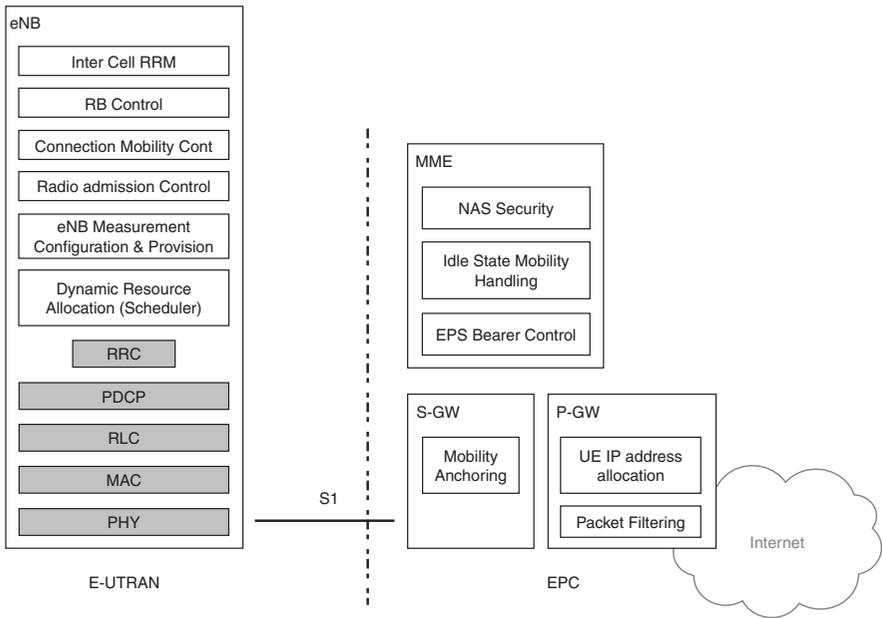
**Figure 9.2** Functional split in LTE and LTE-Advanced. Reproduced by permission of © 2010 3GPP. Further use is strictly prohibited.
