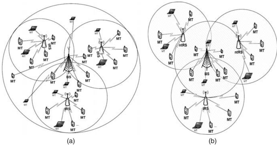
**Figure 3.2** Example deployments of IEEE 802.16-2009 relay networks (i.e., amendment j), with (a) showing tRS and (b) showing ntRS.
