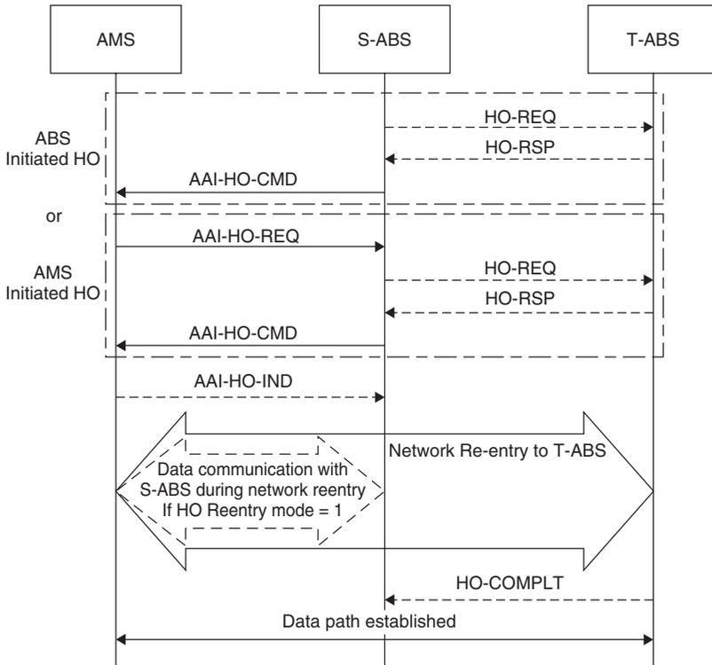
**Figure 3.8** The general handover procedure in IEEE 802.16m. Reproduced by permission of © 2009 IEEE.
