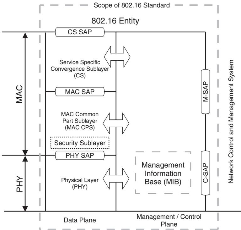
**Figure 3.3** The IEEE 802.16-2009 Protocol Reference Model. Reproduced by permission of © 2009 IEEE.
