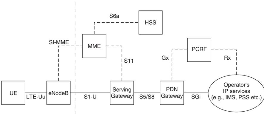
Figure 15.5 LTE Network Architecture.
