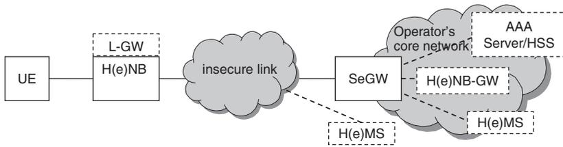
**Figure 9.6** Security system architecture of HeNB.
