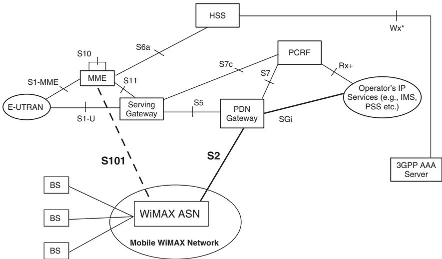
**Figure 16.4** Architecture for optimized handover between mobile WiMAX and 3GPP using L2 Tunneling.
