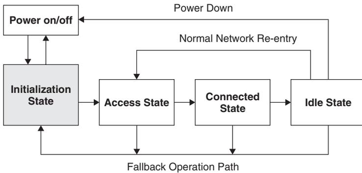
**Figure 5.3** Transitions of an Advanced Mobile Station (AMS).
