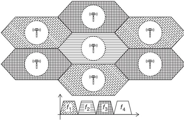
**Figure 2.4** Fractional frequency reuse [4].
