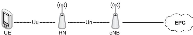
**Figure 12.3** LTE-Advanced-relay architecture: redraw to unify the objects used to represent the UE and eNodeB. Reproduced by permission of © 2010 3GPP. Further use is strictly prohibited.
