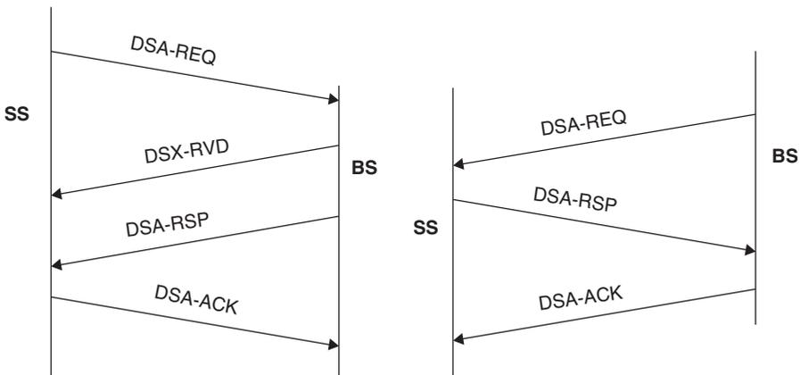
**Figure 6.5** Service flow initiation (a) MS-initiated, (b) BS-initiated. Reproduced by permission of © 2009 IEEE.
