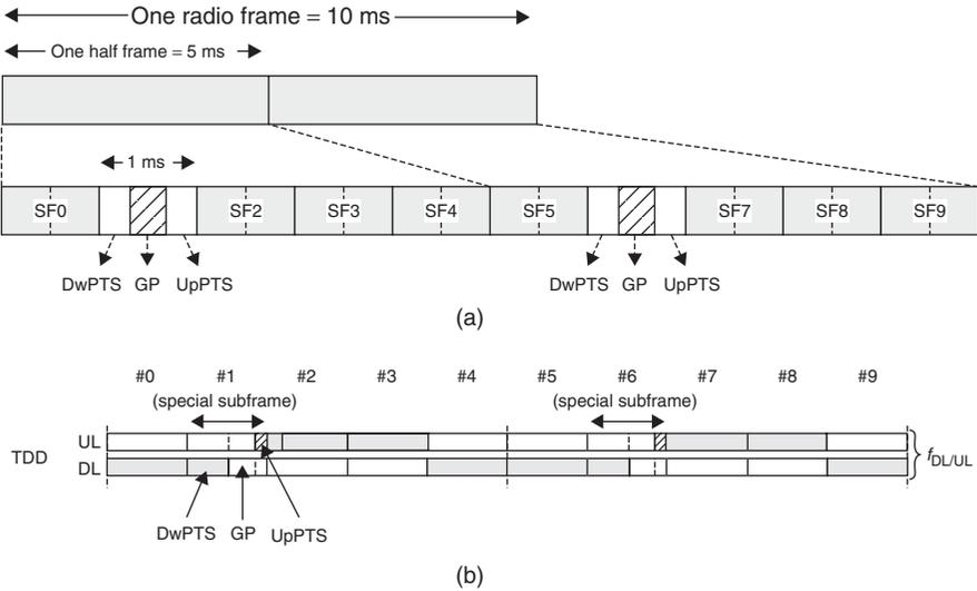
**Figure 10.2** Type-2 Frame structure. Reproduced by permission of © 2010 3GPP. Further use is strictly prohibited.
