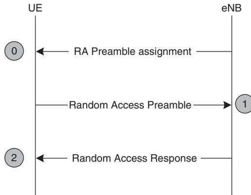
**Figure 11.3** Non-contention based Random Access Procedure. Reproduced by permission of © 2010 3GPP. Further use is strictly prohibited.
