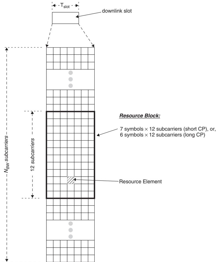
**Figure 15.3** The OFDMA Frame Structure.
