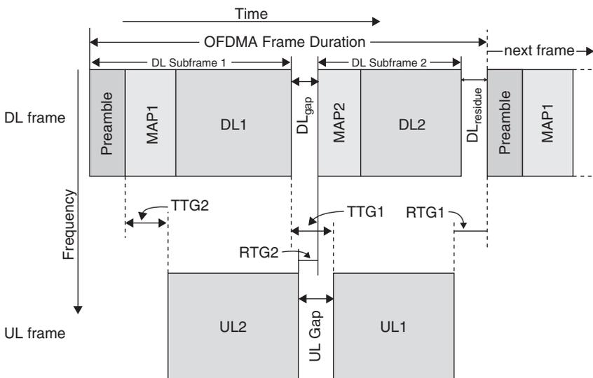
**Figure 4.2** OFDMA and OFDM frame structure FDD operation mode. Reproduced by permission of © 2009 IEEE.
