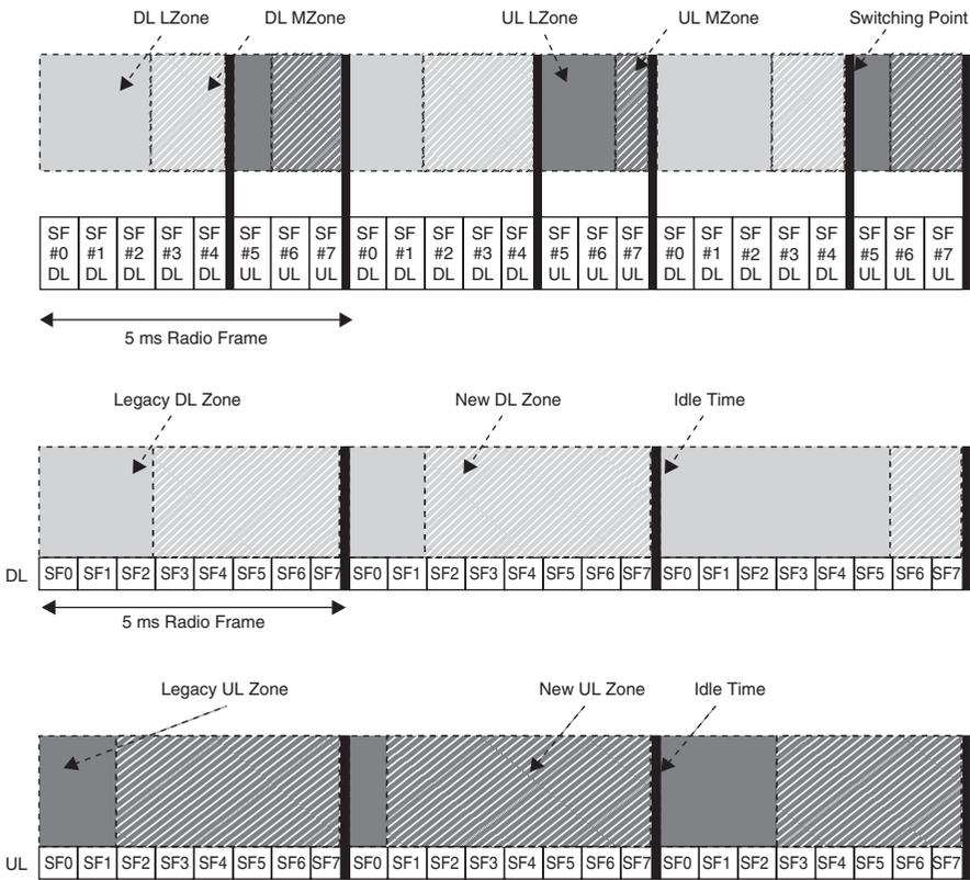
**Figure 4.9** Example of Time zones in TDD and FDD modes. Reproduced by permission of © 2009 IEEE.
