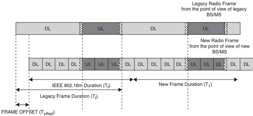
**Figure 4.8** IEEE 802.16m frame structure supporting IEEE 802.16-2009 frames. Reproduced by permission of © 2009 IEEE.
