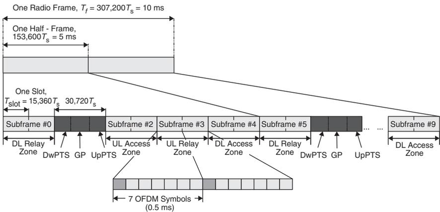
**Figure 10.4** TDD-LTE-Relay frame structure: change to make it similar to the single hop relay structure forma. Reproduced by permission of © 2010 3GPP. Further use is strictly prohibited.
