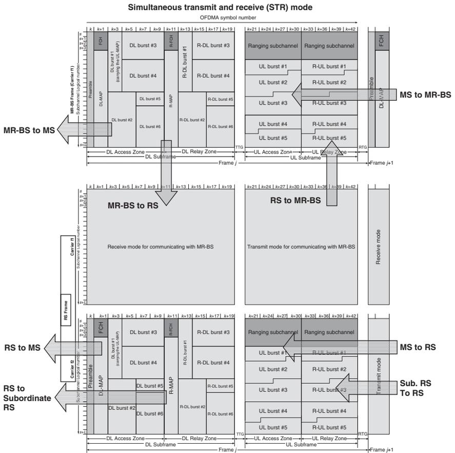
**Figure 4.5** IEEE 802.16j-2009, Part 16: Air Interface for Broadband Wireless Access Systems Amendment 1: Multiple Relay Specification. Reproduced by permission of © 2009 IEEE.
