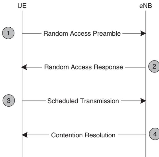
**Figure 11.2** Contention based Random Access Procedure. Reproduced by permission of © 2010 3GPP. Further use is strictly prohibited.
