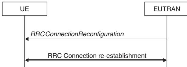
**Figure 11.6** A failure RRC Connection Reconfiguration. Reproduced by permission of © 2010 3GPP. Further use is strictly prohibited.
