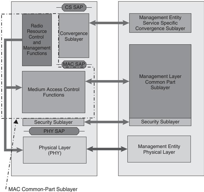
**Figure 3.6** The IEEE 802.16m System Reference Model. Reproduced by permission of © 2009 IEEE.
