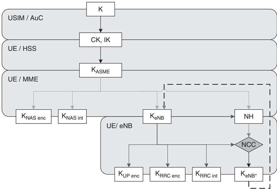
**Figure 14.3** EPS Key Hierarchy and Derivation. Reproduced by permission of © 2010 3GPP. Further use is strictly prohibited.
