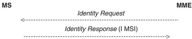
**Figure 10.5** UE unique identification request and response. Reproduced by permission of © 2010 3GPP. Further use is strictly prohibited.
