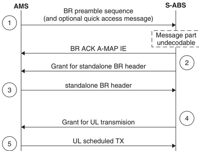
**Figure 3.7** The bandwidth request mechanism in IEEE 802.16m. Reproduced by permission of © 2009 IEEE.
