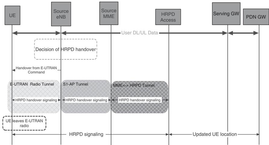
**Figure 16.3** Handover procedure from LTE to CDMA2000.
