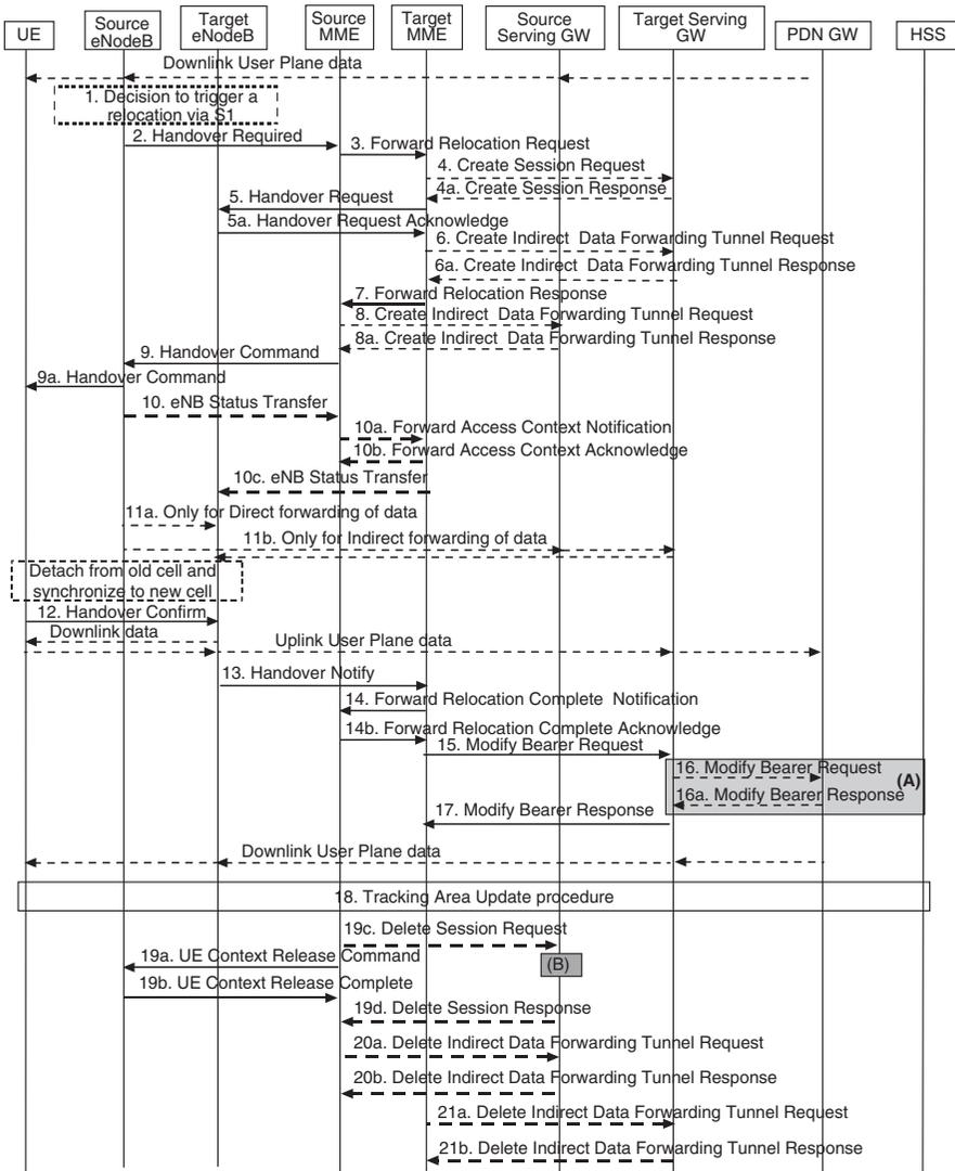
**Figure 13.6** A General S1-based handover. Reproduced by permission of © 2010 3GPP. Further use is strictly prohibited.
